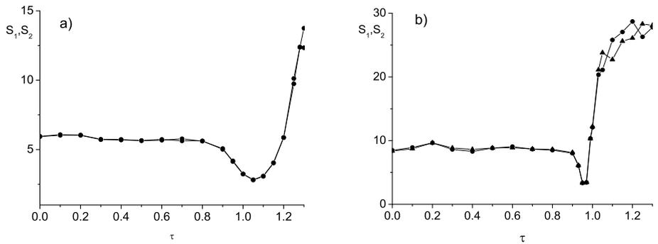
**Fig. 6** Illustrates dependence of  $S_1$  (triangles) and  $S_2$  (circles) on the time-lag  $\tau$  for the values of  $D_1, D_2$  that imply in the maximal SC-SC  $D_1 = 0.0, D_2 = 0.01$  (a) and maximal SISR-SISR  $D_1 = 0.0, D_2 = 0.01$  (b) when there is no time-delay  $\tau = 0$
