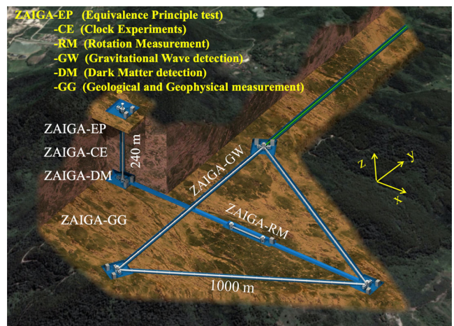
FIG. 22. Layout of the ZAIGA laboratory near Wuhan, China for a range of experiments using atom interferometry. Reproduced with permission from Zhan et al. , Int. J. Mod. Phys D 29 , 1940005 (2020). Copyright 2020 World Scientific Company. 7
