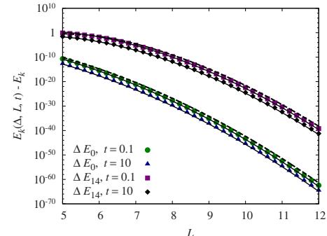
FIG. 7. (Color online) Deviations  $E_k(\Delta, L, t) - E_k$  for a harmonic oscillator as a function of space cutoff  $L$  for different values of time of evolution  $t$ . The parameters used are  $\Delta=0.1$ ,  $\omega=1$ , and  $M=1$ . Solid thin lines give the dominant behavior of Eq. (21). The dashed thick lines correspond to the error estimate in Eq. (18).
