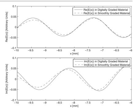
**Figure 3.** Comparison of the electric fields in the initial (smoothly graded) optical potential and the digitally graded optical potential. The initial conditions are the same within the central parts of the structures, so the differences between the approximated and the 'accurate' electric field functions are very small therein. The biggest difference appears at the end of the domain, which is here enlarged for clarity.
