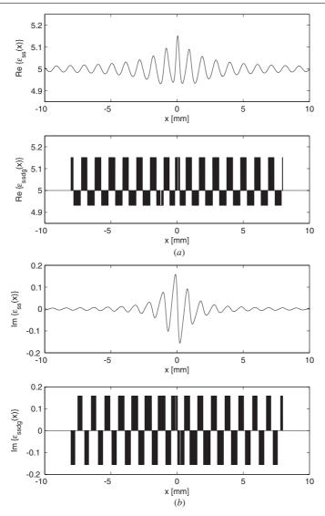
Figure 4. The results of the digital grading approximation with three values for both (a) the real and (b) the imaginary part.
