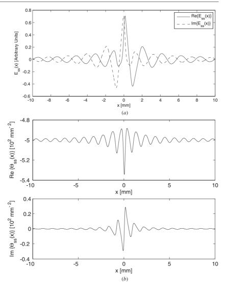
Figure 1. (a) An example of the supersymmetric localized electric field; (b) the corresponding supersymmetric optical potential, for C=3+3i,  $\rho=6$  mm, k=3 mm<sup>-1</sup>,  $k_0^2 \varepsilon \mu=500$  mm<sup>-2</sup>.
