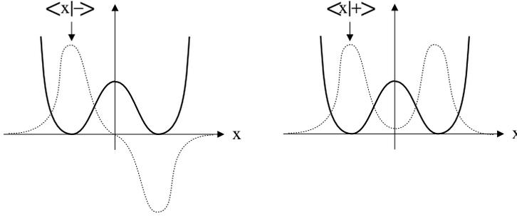
Figure 18.5: The double well and its two lowest eigenstates
