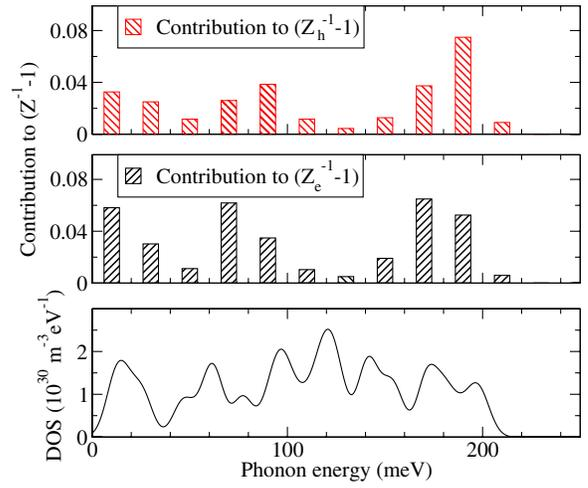
FIG. 3 (color online). Upper panel: Contributions of different phonon modes, divided into 20 meV-wide energy intervals, to the quasiparticle renormalization for electrons and holes. Lower panel: Phonon density-of-states (DOS).
