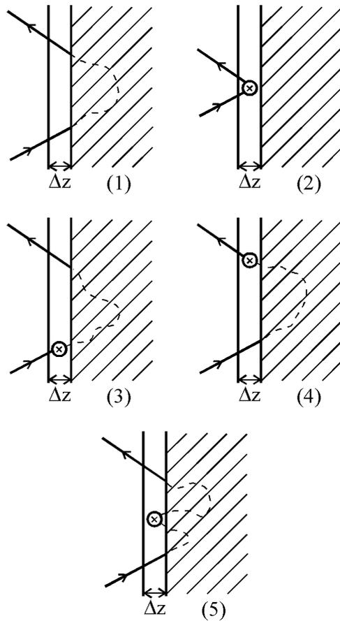
**Figure 1.** Relevant events in the thin layer during the reflection of a photon. The crosses denote single scattering in the layer while the broken lines represent backscattering in the infinite medium.
