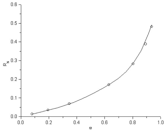
**Figure 3.** Total reflection coefficient for normal photon incidence as a function of the parameter  $\omega$ . Comparison of the Monte Carlo results (circles) with analytic theory (full line).
