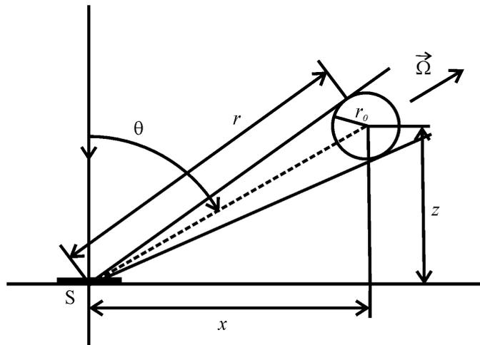
Figure 5. The scheme of the scattering geometry.
