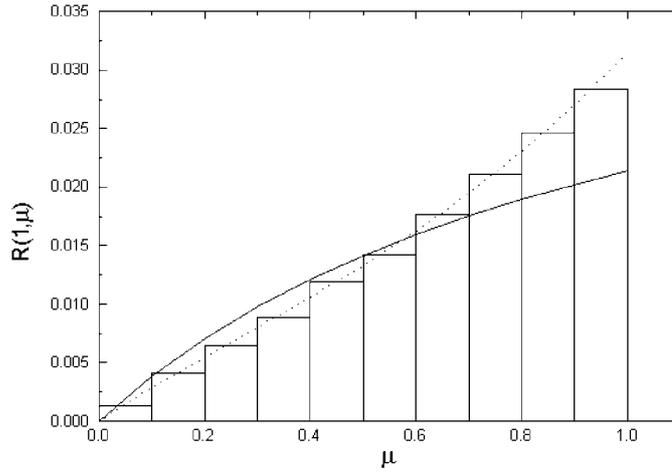
**Figure 4.** Angular distribution of backscattered photons for photon incident energy  $E = 10$  keV. (—) Results from isotropic model. (·····) Results with the single backscattering anisotropy included. Histogram from the Monte Carlo simulation.
