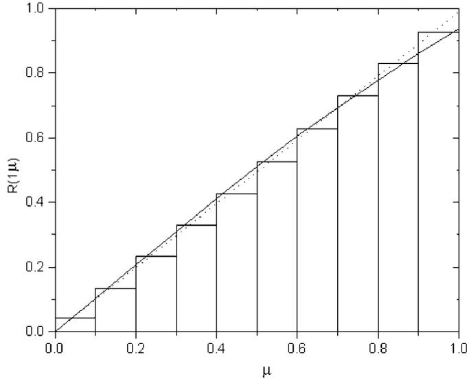
**Figure 2.** Angular distribution of backscattered photons at normal incidence for photon energy  $E = 60$  keV. (—) Results from isotropic model and (·····) results from cosine distribution. The histogram is from the Monte Carlo simulation.
