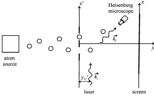
**Figure 1.** The scheme of Feynman's atomic microscope. After passing through a grating, atoms undergo resonance scattering with photons from a laser beam parallel to a grating at a distance  $y'_{12}$ . Atoms are detected at the screen at the distance  $y$  from the grating.
