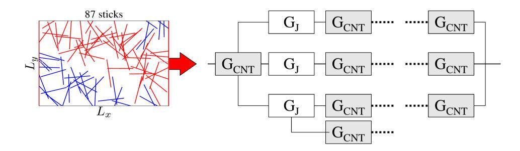
CNT is replaced with resistor network
