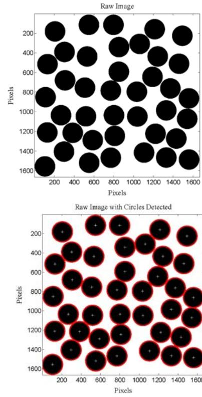
**Figure 3.** Two-dimensional system of disks from numerical simulation (left); detection of the disks' circumferences and associated centres (right).
