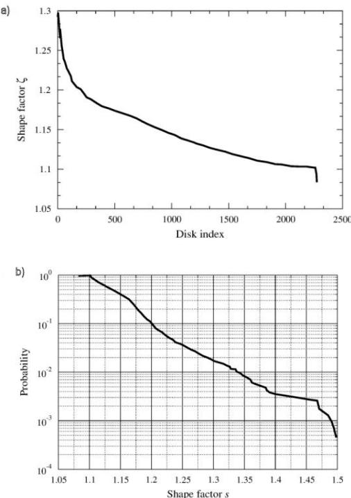
**Figure 10.** (a) Values of the shape factor for all Voronoï polygons, for the same disks configurations as in Fig.7; (b) The probability that the value of the shape factor  $\zeta$  is greater than  $s$
