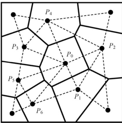
**Figure 1.** The “perpendicular bisector method” for constructing the Voronoï diagrams in 2D
