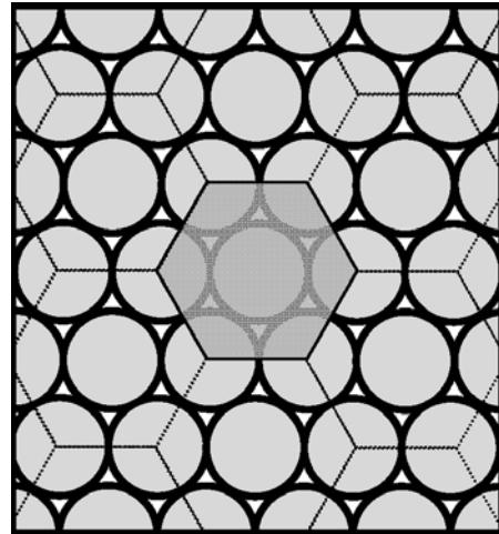
**Figure 2.** Two-dimensional hexagonal package of equal disks. Disk centres are vertices of regular hexagons
