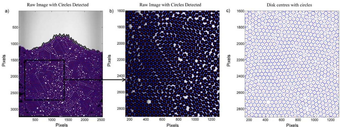
**Figure 6.** CHT analysis of the packing at density  $\rho=0.79$ : (a) The whole domain; (b) A part of the same snapshot with the centres. (c) Extracted disk centres and circles
