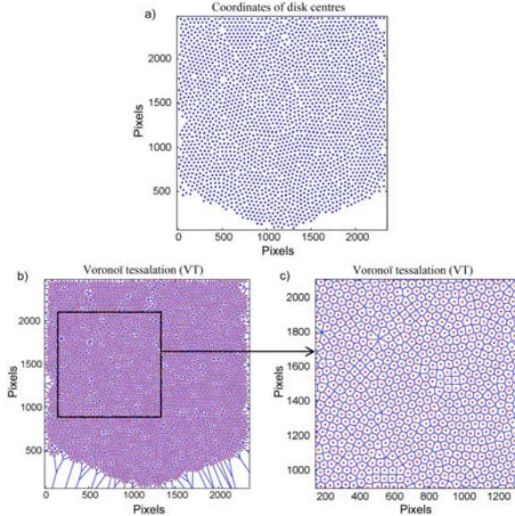
**Figure 7.** Voronoi tessellation of a set of point particles (centres of disks). Diagrams correspond to the experimentally obtained packing at density  $\rho=0.79$ : (a) Centres of disks; (b) Voronoi diagram; (c) The part of the same diagram. The centres of grains are marked with dots
