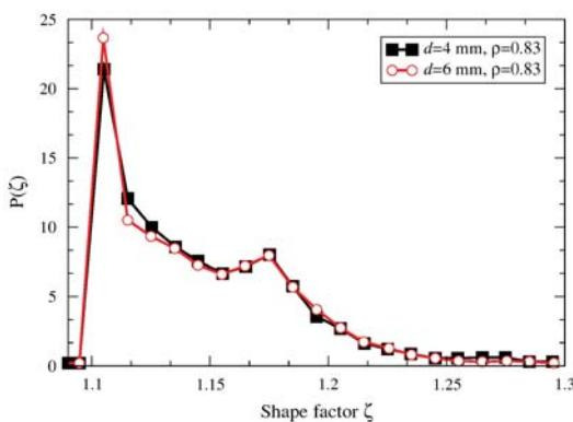
**Figure 11.** Experimental results for the probability distribution  $P(\zeta)$  of the shape factor  $\zeta$ . The experimental results correspond to the packings of disks of diameter  $d=4$  (□) and  $6$  (○) mm at density  $\rho=0.83$ .
