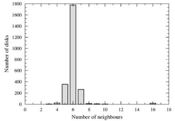
**Figure 8.** Distribution of Voronoï neighbours for packing shown in Fig.7. The number of opened cells located on the boundaries are also indicated as number of cells with  $n_c = 16$  edges.
