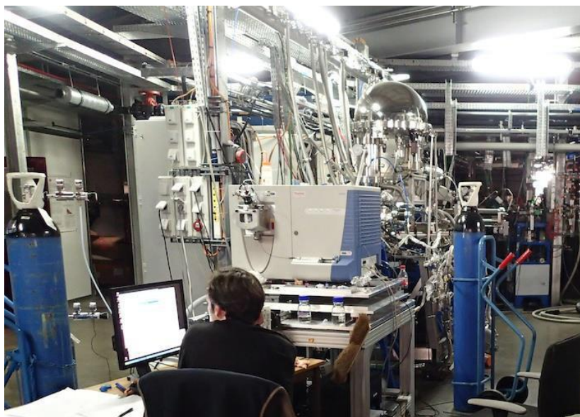
Figure 2.9: A photo of the experimental setup – coupling the LTQ XL mass spectrometer mounted on a dedicated supporting frame with the PLEIADES beamline at the SOLEIL synchrotron facility.
