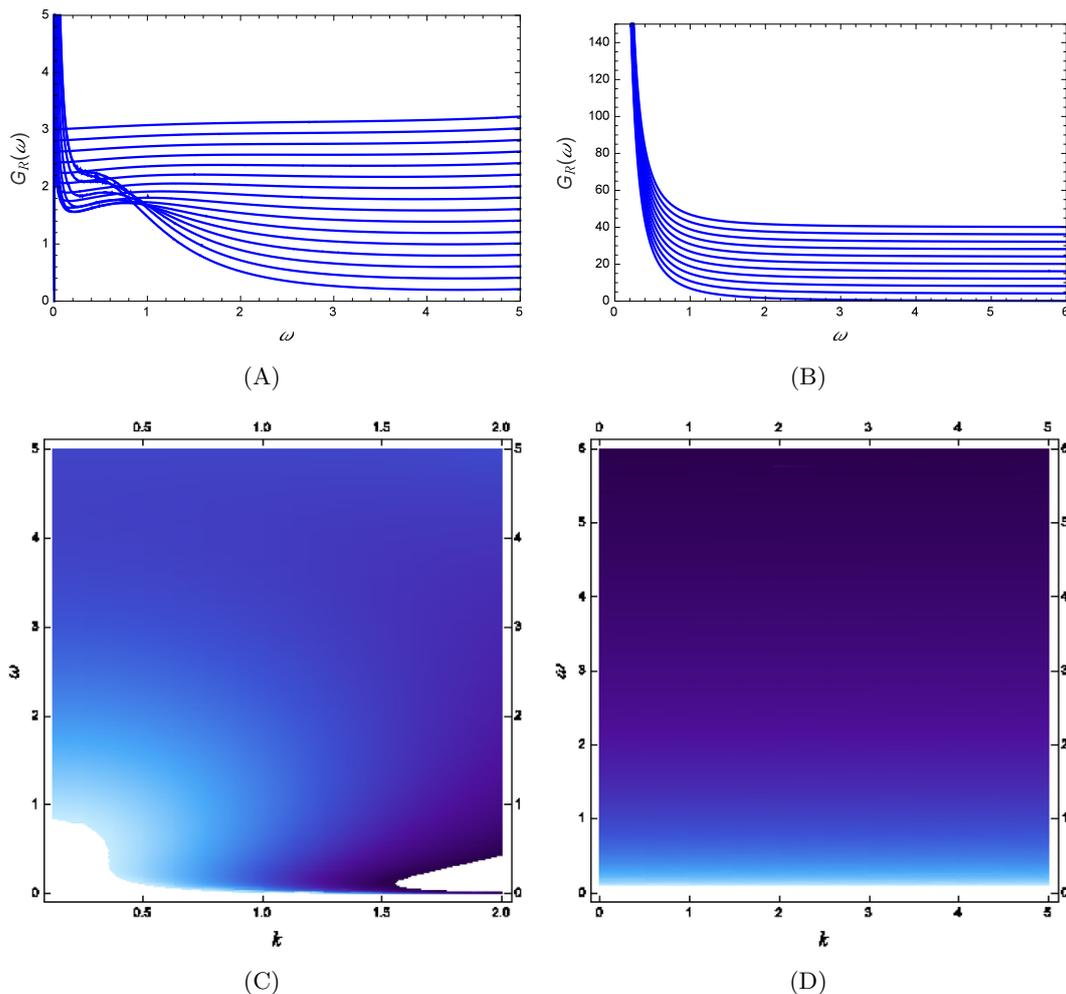
**Figure 11.** The retarded propagator  $\Im G_R(\omega)$  in the confined/non-condensed phase (A,C) and in the deconfined/condensed phase (B,D) in a neutral system. While the deconfined case is again an almost exact power law, the confined case has a scale but no quasiparticle. The discrete  $Z_2$  symmetry has no zero modes upon breaking. The retarded propagator is thus not so useful when the system is neutral.
