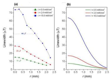
Fig. 4. Experimental (a) and theoretical (b) Hanle EIT linewidths for the different positions r of the aperture along the laser beam diameter. The blue, the red, and the green curves are for the intensities  $I = 15 \text{ mW/cm}^2$ ,  $2 \text{ mW/cm}^2$ , and  $0.5 \text{ mW/cm}^2$ , respectively. The dashed bars in (a) represent the Hanle EIT linewidths obtained by detecting the whole laser beam.
