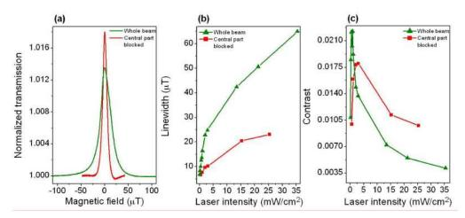
Fig. 5. (a) The experimental Hanle EIT resonances obtained when the whole beam is detected (green curve) and when the central part of the beam is blocked in front of the detector (red curve). In (b) and (c) linewidth and contrast of the EIT versus laser intensity are given for the whole beam (green) and for the beam with blocked central part (red). The central part was blocked by circular mask of diameter d = 2.2 mm. The laser intensity is 3 mW/cm<sup>2</sup>.
