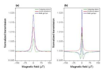
Fig. 3. Calculated contribution of outgoing (green), incoming (red) and both outgoing and incoming (blue) atoms to the Hanle EIT resonances for two distances from the laser beam center: r = 1.00 mm (a) and r = 1.75 mm (b). The total laser intensity is  $3 \text{ mW/cm}^2$ .
